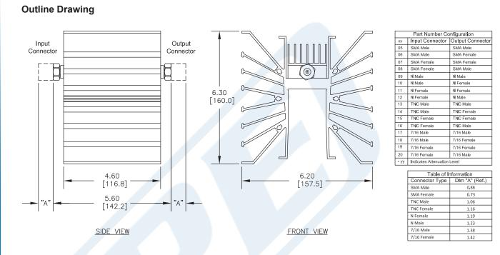
6 dB Fixed Attenuator, SMA Male To SMA Male Directional Black Aluminum Heatsink Body Rated To 300 Watts Up To 3 GHz from Pasternack Enterprises has same day shipment for domestic and International orders. Our RF, microwave and millimeter wave products maintain a 99% availability and are part of the broadest selection in the industry.
